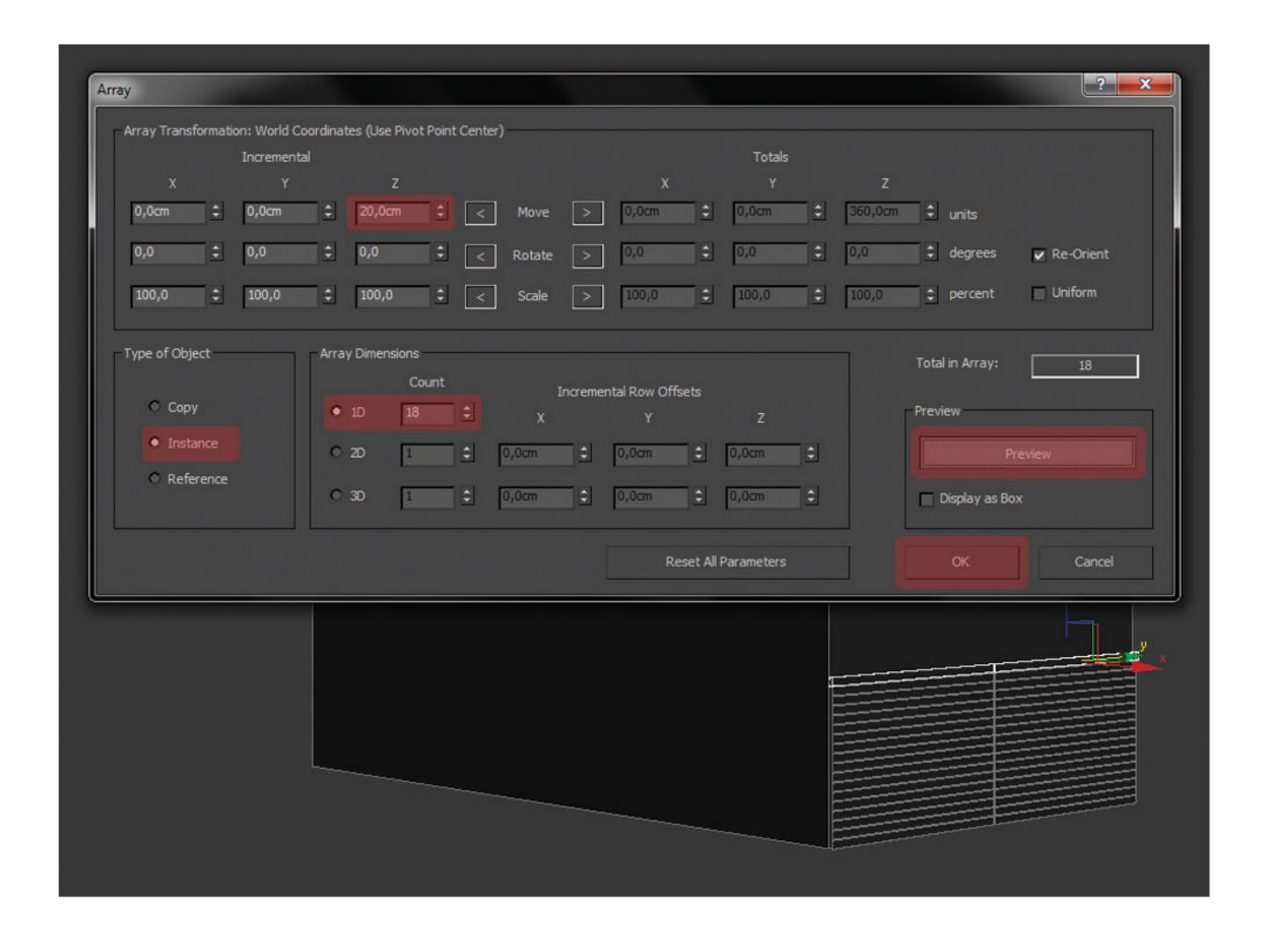
The second step of three - modeling of the midle elements (curved horizontal elements). We will do again previous *Array* operation, but with 50 pieces.
